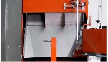
The Javo Plus M2.0 is suitable for 10 up to 32cm pots. The potting machine is available in different pot track configurations, each for its own purpose. Apart from the standard configuration with adjustable tray support, it is also possible to provide the pot track with a barerootsystem. Adjustable chutes bring substrate onto a flexible plate behind the pot, for the possibility to put extra soil in the pot. This is truly a versatile potting machine.
