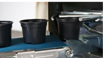
This small, strong potting machine is a workhorse suitable for pots from 8-21 cm. The fast, easy central adjustment allows for quick, perfect changes between pot sizes. The Ecobasic is technically advanced and extremely mobile, allowing for easy relocation. The machine includes a mechanical pot dispenser, pot take off, drill installation and a conveyor belt with variable speed. The takeoff for the pots onto the conveyor belt can be positioned to the left, right and front of the pot track.
