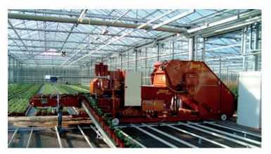
This dosing unit handles substrate or bark from all full-size compressed bales with ease. The powerful motor-driven tilting system allows a big bale to be tilted into place efficiently and safely while keeping the work environment clean.
