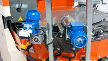
The Javo Plus has 16 pot positions and is suitable for 9-23cm pots. The machines in the Plus series are characterized by the round pot track, suitable for round and (optional) square pots. Like the other members of the Plus family, the Plus uses a fast,
