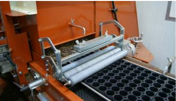
This extremely reliable and unique tray filling machine processes various types of trays, including plug trays and multi-cell trays.
